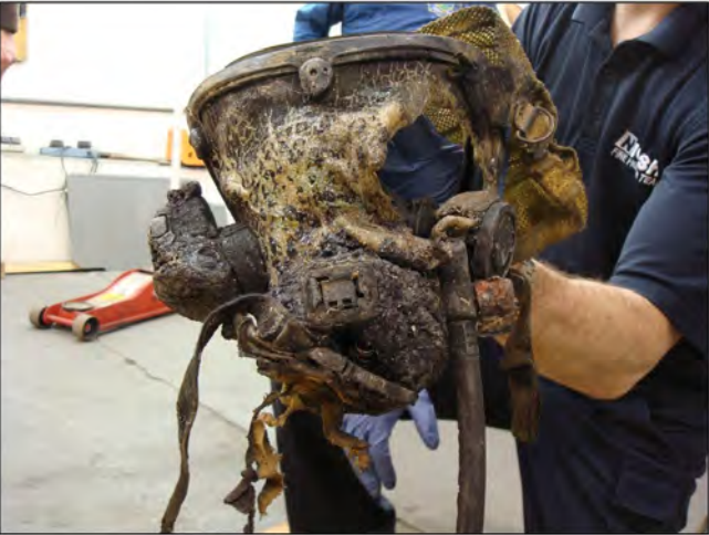
Photo 1. Victim's melted facepiece lens. (NIOSH Photo.)
