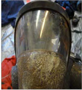
Photo 4. FF2's facepiece showing thermal degradation. (NIOSH photo.)
