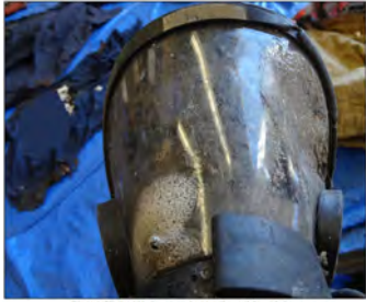
Photo 1. Victim 11's facepiece showing thermal degradation. (NIOSH photo.)
