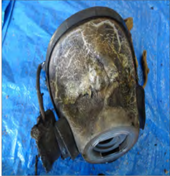
Photo 3. FF1's facepiece showing thermal degradation. (NIOSH photo.)
